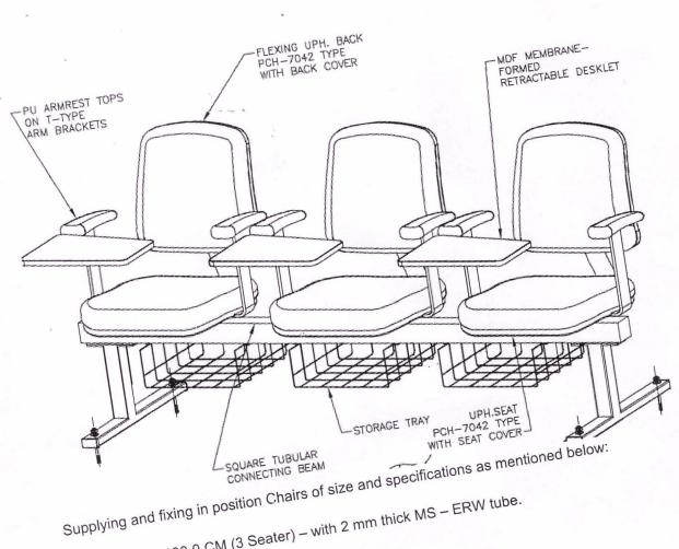
Overall Width: 190.0 CM (3 Seater) - with 2 mm thick MS - ERW tube.
